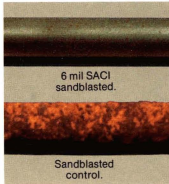
Pipes after three-year burial test.
