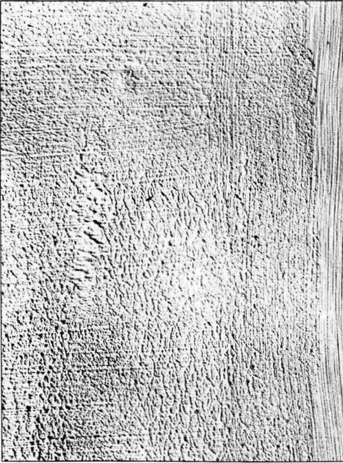
Figure 9—Typical panel from first series of tests evaluating color acceptance of test paint in side-by-side brush and roller applications
