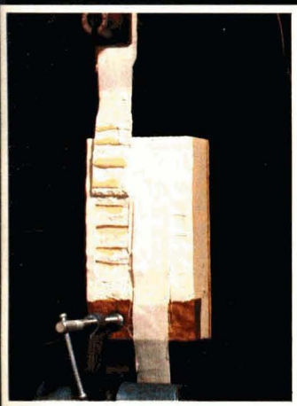
The foam actually tore during peel adhesion testing on an Instron unit documenting adhesion of the mastic based on RHOPLEX EC-1791 acrylic.
