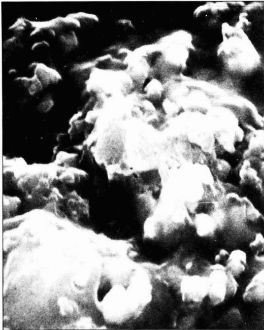
Figure 2A—Micrograph (1000 X) of latex coating with chlorothalonil following 400 hrs exposure in accelerated weathering device
