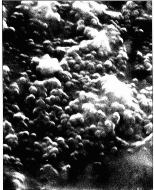
Figure 2B—Micrograph (1000 X) of latex coating following 400 hours exposure in accelerated weathering device
