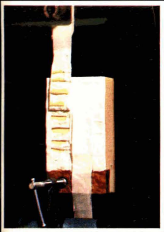
The foam actually tore during peel adhesion testing on an Instron unit documenting adhesion of the mastic based on RHOPLEX EC-1791 acrylic.
