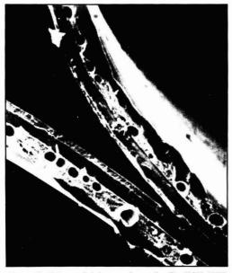
Figure 16—Entrapped air in a powder coating film (SEM, 100X)
