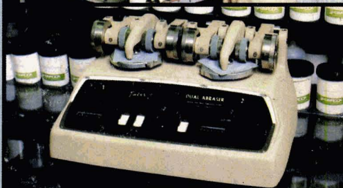
TOP: Reactor produces developmental polyethylene waxes. MIDDLE: Samples are prepared by roller, brush, draw-down and spray application techniques. BOTTOM: Testing is conducted for slip and friction, rub and mar, and wear and abrasion.*
