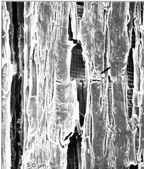
Figure 5—SEM photo of xylene-borne alkyd panel after 555 hours of weathering. Note openings (cracks) up to 100 \mu\text{m} wide. Arrows point to two cross-grain checks
