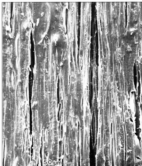
Figure 3—SEM photo of brush-coated xylene-borne alkyd on Eastern white pine after 267 hours of accelerated weathering
