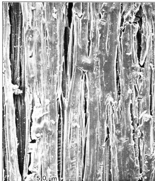
Figure 6—SEM photo of water-borne alkyd panel after 555 hours of accelerated weathering has narrower checks; arrows point to two cross-grain checks
