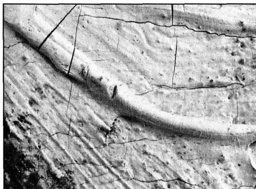
Figure 8—Photomicrograph of a cross-sectioned cut made through a ridge of faded pink paint found in a modern oil painting. The white faded portion at the top and the unfaded pink below illustrate clearly that fading occurs in layers. Magnification is about 10 diameters
