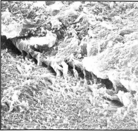
Figure 6—Scanning electron microscopy photograph of the transition from zone (ii) to zone (iii) failure on the steel sheet (see text)
