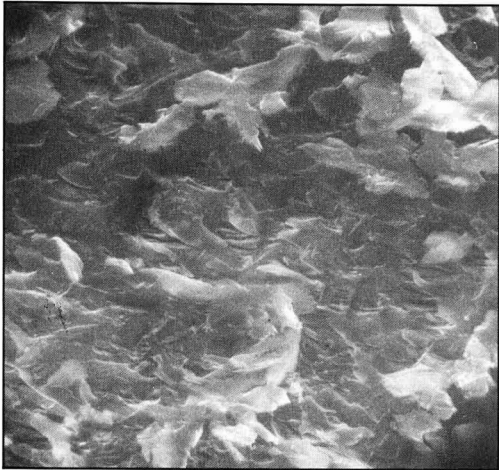
Figure 1—SEM photograph of failure surface (cylinder) of the Z2 system
