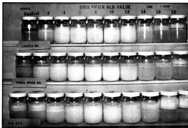
Figure 4—A display illustrating the HLB evaluation of three components (standard mix ratios). The components are oils at 100% (no diluent solvent used). The top row set contains linseed oil, the second row set contains china-wood oil, and the bottom row set contains GH dehydrated castor oil. The sets are shown 1 hr after agitation
