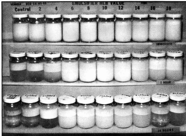
Figure 1—A display of the HLB evaluation of component G-H dehydrated castor oil with mineral spirits/66 as diluent, illustrating the degree of emulsification remaining at three separate time frames. The emulsification achieved immediately after agitation is illustrated by the top row set for a control (no emulsifier) and the HLB series 2-18. The second row set illustrates the degree of emulsification remaining one hr after agitation. The bottom row set illustrates the remaining degrees of emulsification for the HLB series after 24 hr
