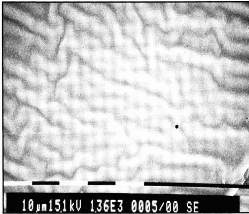
Figure 11—Micrograph of IPN-1 coating [90/10 P(EU)-1/P(UA)-1]
