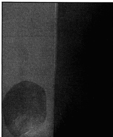
Figure 1—Rub up of acrylic latex enamel. Left—control; right—wetting agent
