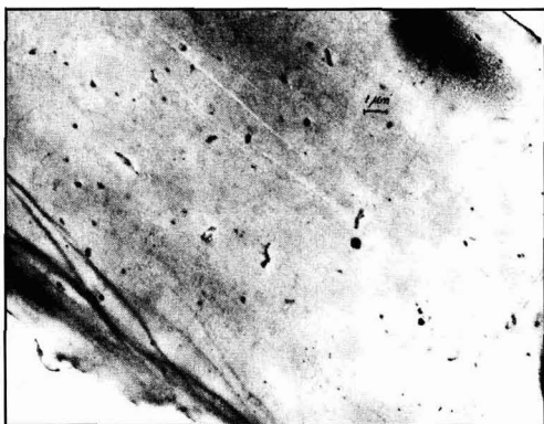
Figure 2—The same plastisol as in Figure 1, but completely gelled to form a continuous film. Single PVC-particles can no longer be seen but for a few pigment particles. Approximately 6000x
