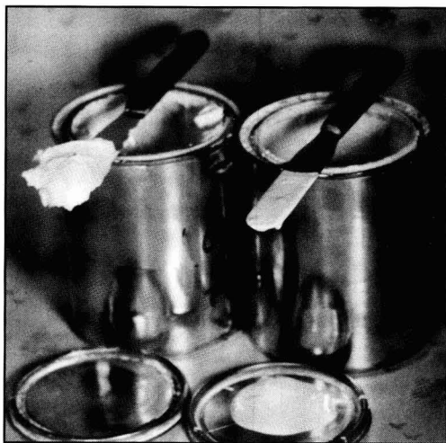
Figure 4 — Differences in flow properties due to degree of dispersion for the same pigment
