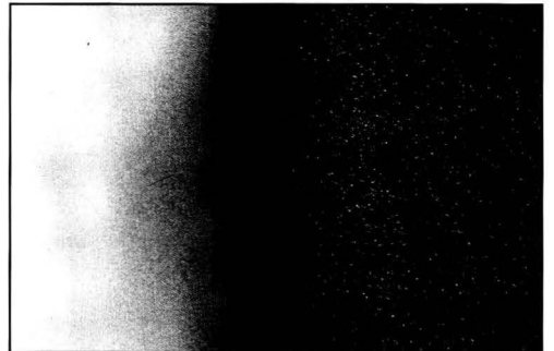
Figure 7—Light microscopic view of a drop of flocculated paint (right) coming into contact with a drop of paint containing blanc fixe HU (left)
