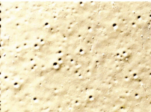
Airless sprayed waterborne maintenance coating with Surfynol additives on metal test panel (15x mag.).
