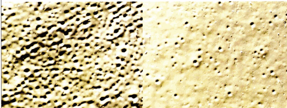
Standard airless sprayed waterborne maintenance coating on metal test panel (15x mag.).
