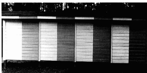
Figure 3—White and gray test paints and controls applied two coats over latex primer on southern yellow pine, exposed on test wall at south vertical in Huber, GA.
