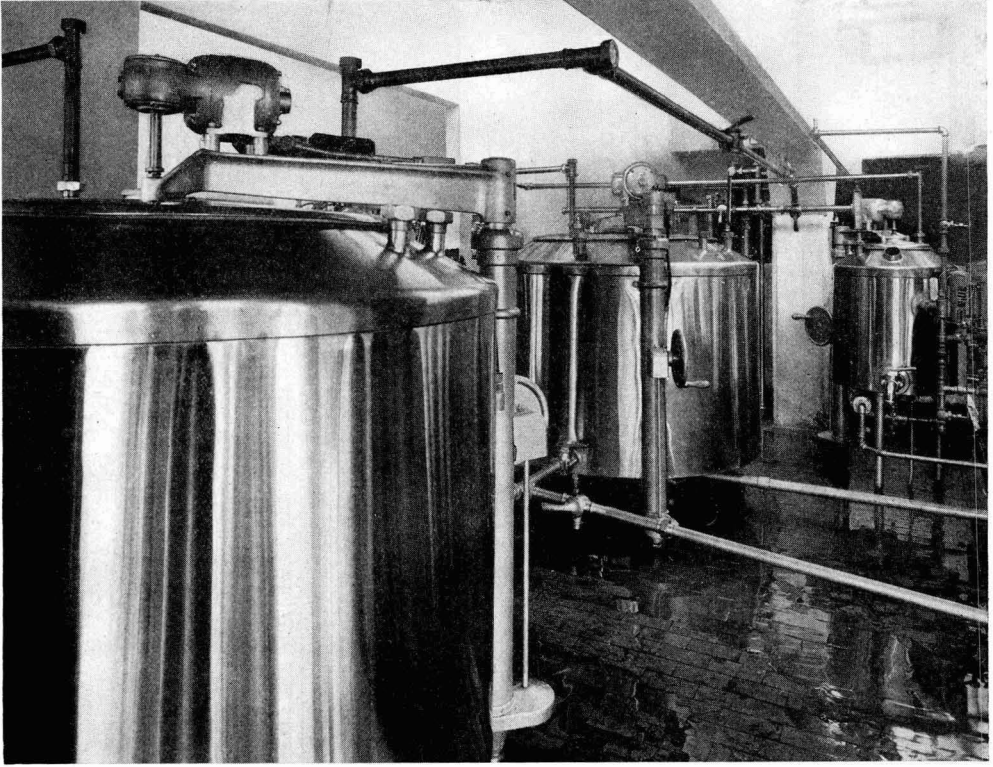
These three Jensen Vacuum "A & G" Machines are operating in Scott-Powell's Philadelphia plant. The two 500-gallon size are used for buttermilk—the 50-gallon size for starter.
