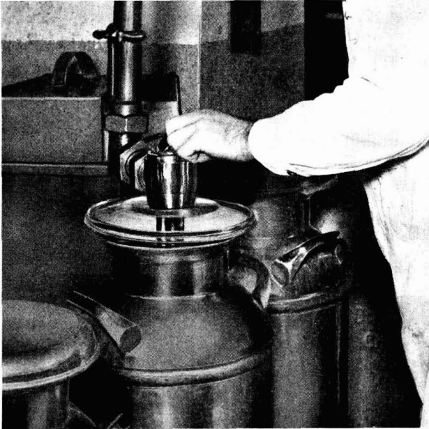
Left: Mojonnier Sanitary Can Filling Plastic Cover in operation.
