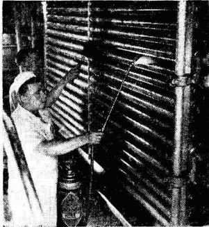
Spraying cooler with cleaning solution to loosen and remove accumulation of milk solids and fats.
