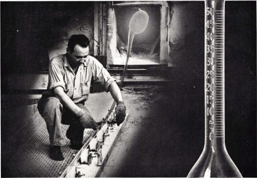
Gauging diameter—a control measure on machine-drawn glass tubing.
