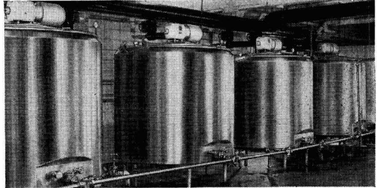
Four 1,000 gallon Mojonnier Zone-Control Vats processing buttermilk. Borden Dairy Co., Detroit.
