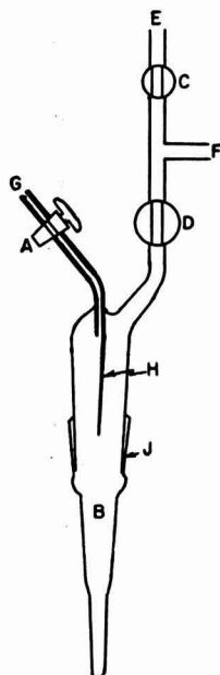
FIG. 1. Modified reflux regulator and sample receiver for Todd fractionation assembly. A—reflux regulator, B—graduated sample receiver, C—2-way stopcock, D—3-way, oblique bore stopcock open at top, E—to McLeod Gauge and top of distillation column, F—to vacuum, G—to distillation head, H—“finger” to direct distillate into center of sample receiver, J—24/40 S/T joint.
