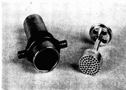
FIG. 1. One type of immobilizing insert used with the laboratory centrifuge. Length of holes, 1.24 cm.; diameter, 0.231 cm.
