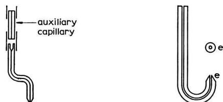
Fig. 3a. End tube C_g provided with auxiliary capillary. Fig. 3b. End tube B_g with edge e at its tip.
