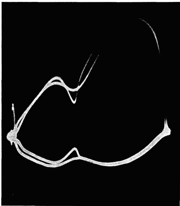
Fig. 2. Comparative measurement: dE/dt = f(E) curves of polyphosphate P_{114} , 3.3mg/ml, and pure electrolyte 1 N H_2SO_4 ; Q = 0.43 .
