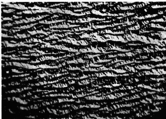
Fig. 7. Ridge-type deposit at 5 mA/cm<sup>2</sup> from a solution containing 10<sup>-7</sup> mole/l of *n*-decylamine.
