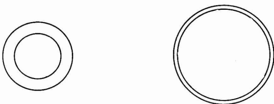
Fig. 1. A concentrically growing Hg drop (inner sphere) plus a constant volume of surrounding solution (outer sphere), at different stages in drop life.
