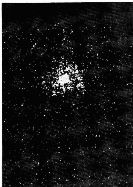
Fig. 4. Sample current pattern obtained with an electron microprobe for a Cu deposit of 1390 \mu\text{C} (deposited under exactly the same conditions as the film which gave the stripping curve illustrated in Fig. 3). One division on the photograph scale represents 18.5 \mu .
