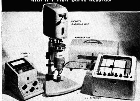
This laboratory instrument is a cone and plate viscometer of advanced design which enables the flow behaviour of many types of simple or complex fluids to be examined.
