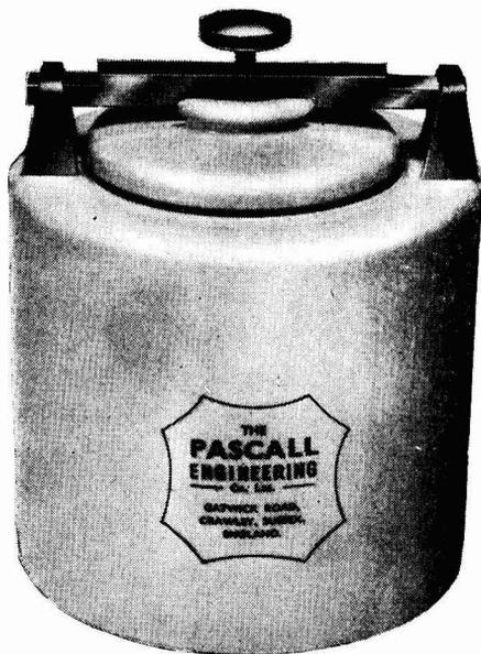
These new type ball mill pots with flat ground tops and flat ground interchangeable covers are already popular with a large number of satisfied users. Made of hard porcelain with the excellent properties of resistance to corrosion and abrasion and freedom from contamination. Ideal for dry or wet grinding ceramic colours, paints and printing inks.
