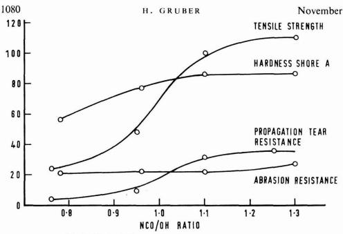
Fig. 2. Mechanical properties of solvent-free polyurethanes
