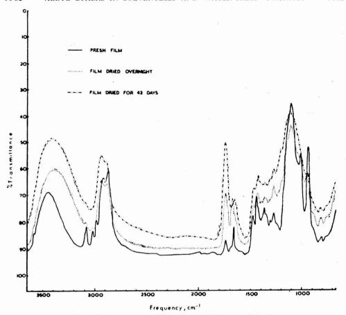
Fig. 2. Infrared spectra of films of sorbitol tetra-allyl ether
