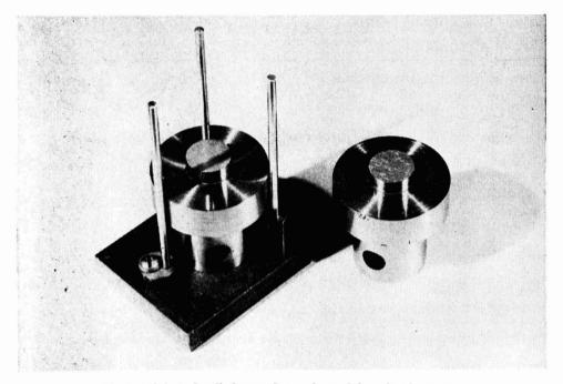
Fig 1. Mild steel cylinders and test rig used for adhesion tests.
