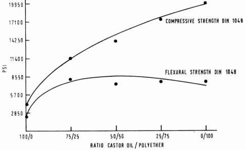
Fig. 6. Mechanical properties of polyurethanes
