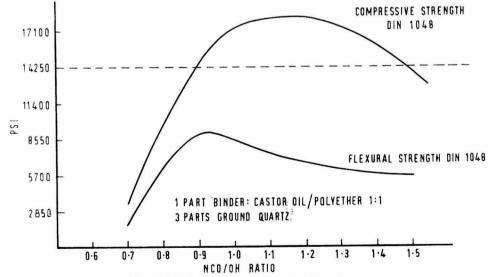
Fig. 7. Mechanical properties of polyurethanes
