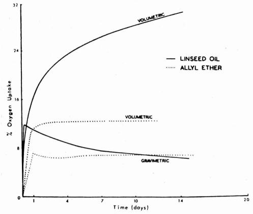
Fig. 1. Oxygen uptake of linseed oil and sorbitol tetra-allyl ether
