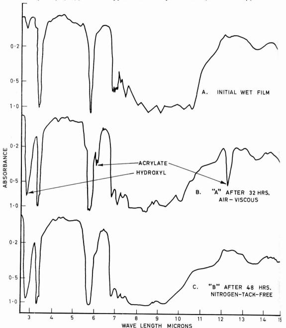
Fig. 9. Oxidation of V-54 sebacate—infrared spectrum
