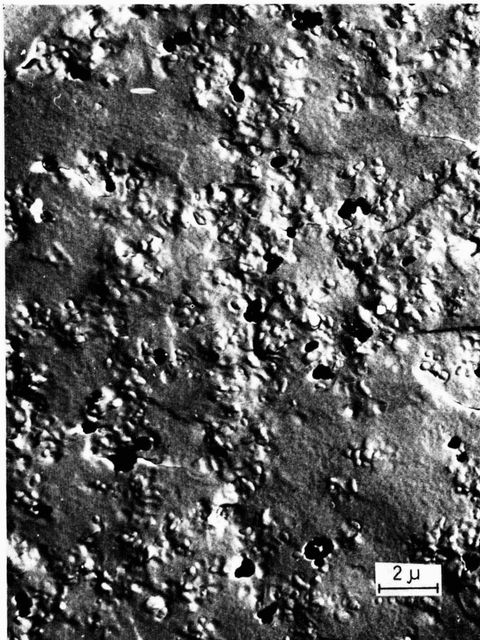
Fig. 18. Fracture surface of a plasticised polybutyl methacrylate film pigmented with titanium dioxide (rutile) (PVC=20)
