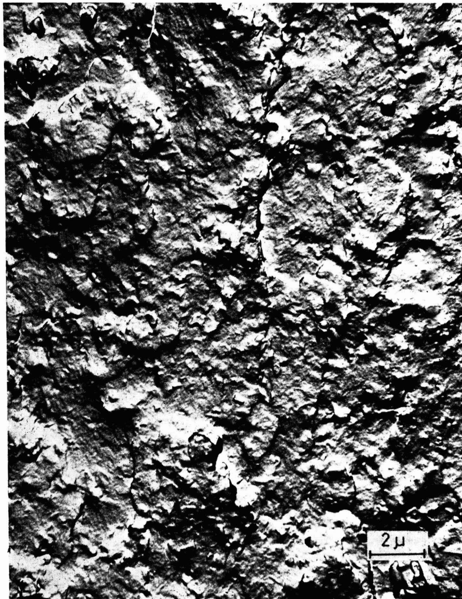
Fig. 15. Fracture surface of an urea formaldehyde resin film pigmented with zinc oxide (PVC=15)
