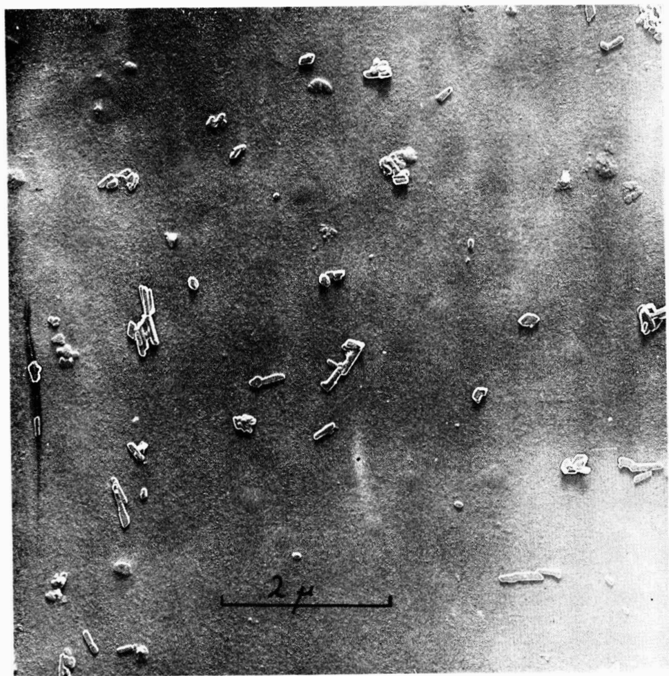
Fig. 2. Electron micrograph of CI Pigment Yellow 1. Replica shadowed at 30°. (By courtesy of P.R.S.)
