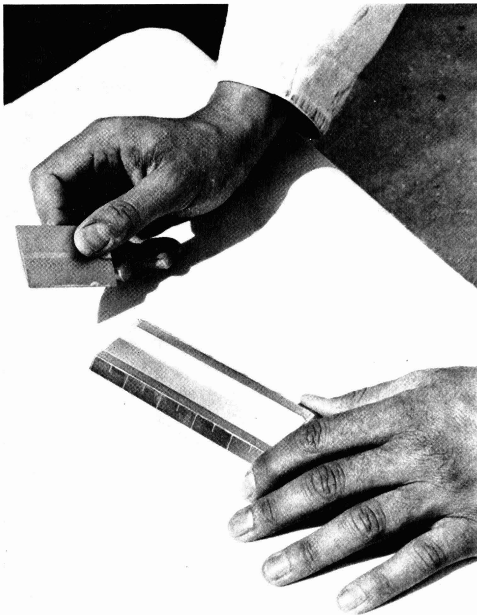
Fig. 2. The opacity gauge in use, showing an opacity reading of 90 microns
