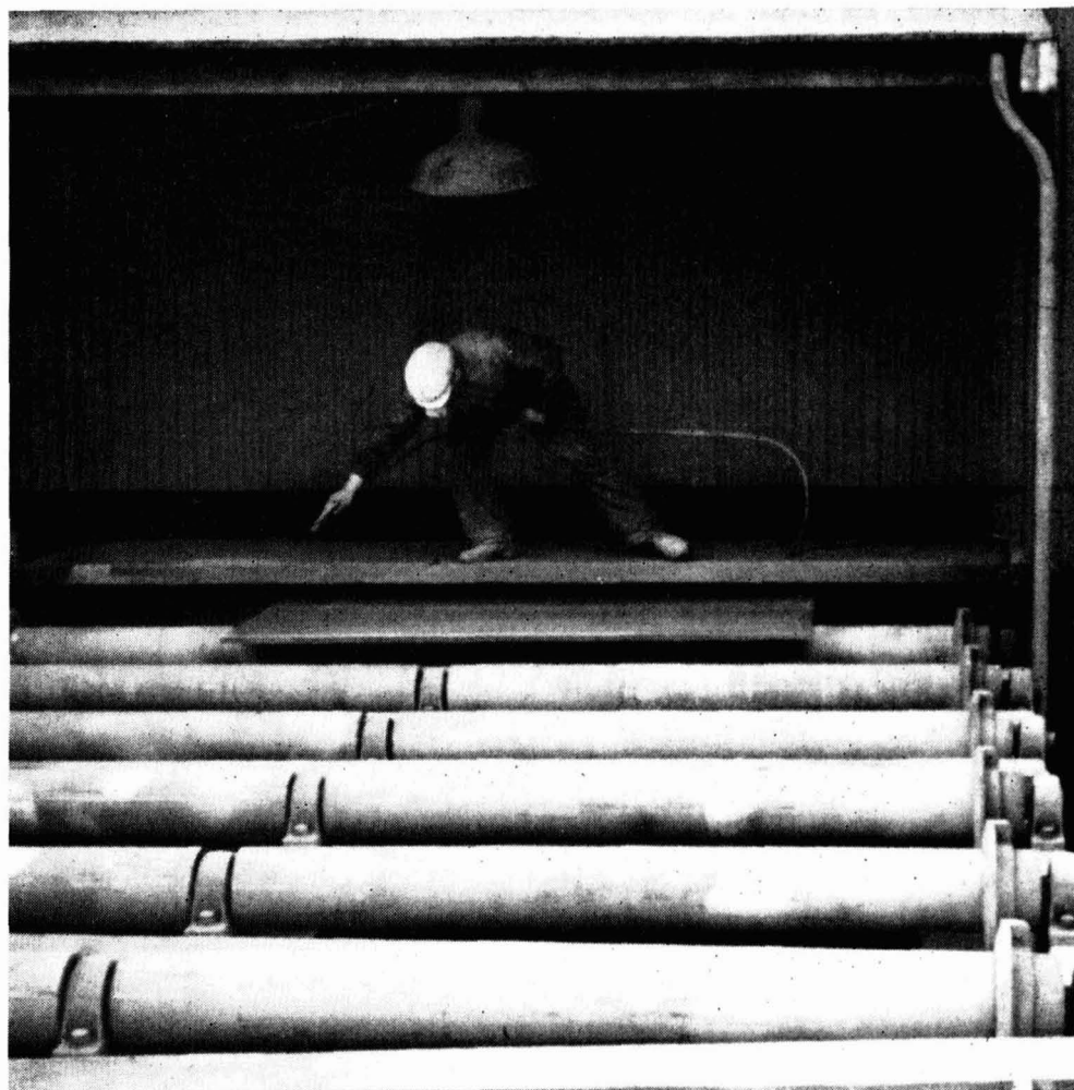
Fig. 3. Incorrect practise in hand spraying
