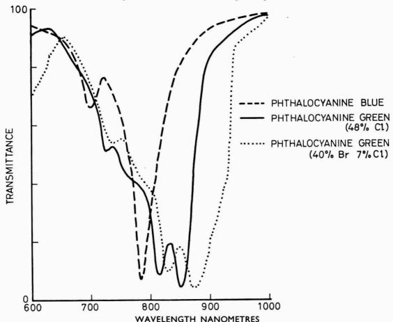
Fig. 1. Absorption curves for phthalocyanine pigments
