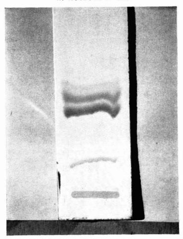
Plate 1—Pigments from printing ink. Developing solvent chloroform/xylene; 3/1. In order of increasing Rf the pigments are 2B toner (Pigment Red 48), Carmine FBB (Pigment Red 146), Red RL (Pigment Red 10), Orange G (Pigment Orange 13), Xylidide Benzidine Yellow (Pigment Yellow 13)
