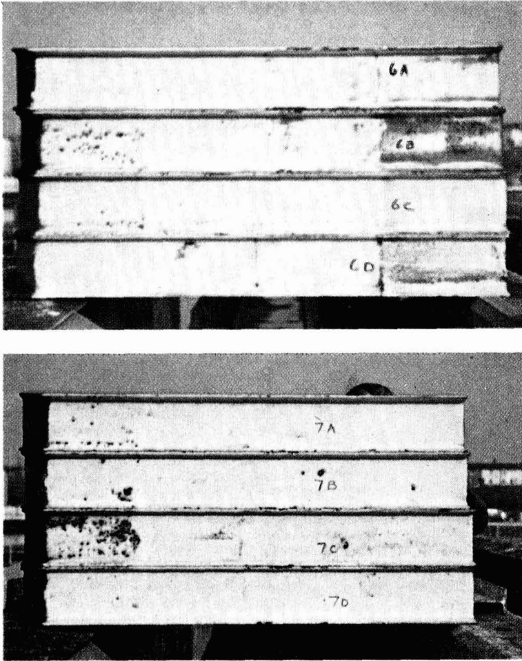
Fig. 8 (top). Exposure of holding primer CEGB 6 before overpainting. From left to right: 12 months, six months, two months, one day. Total exposure of girder three years six months
