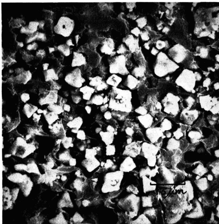
Fig. 5. Film containing 34 per cent cuprous oxide by volume, vertical cross-section
