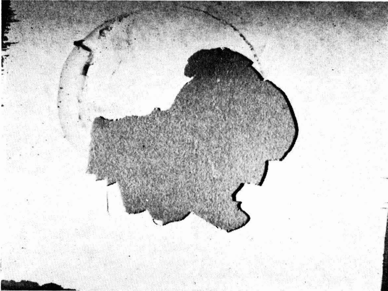
Fig. 15. Internal adhesion failure of System 1, etch primer/chlorinated rubber, on mild steel. Mag. \times 4
