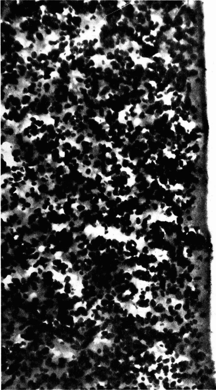
Fig. 1. Section of gloss paint film showing the structure of the paint/air interface
