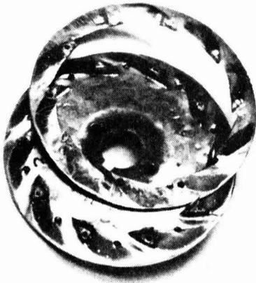
Fig. 8. Worn multi-ring impeller, disassembled, showing wear pattern
