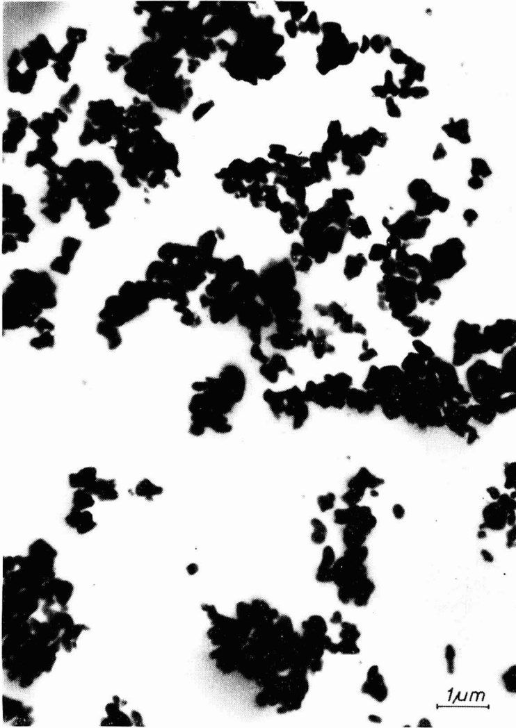
Fig. 5. Part of a cross-section ( \times 11,700 ) of an epoxy resin/ \text{TiO}_2 film ( \lambda_p = 0.1 )
