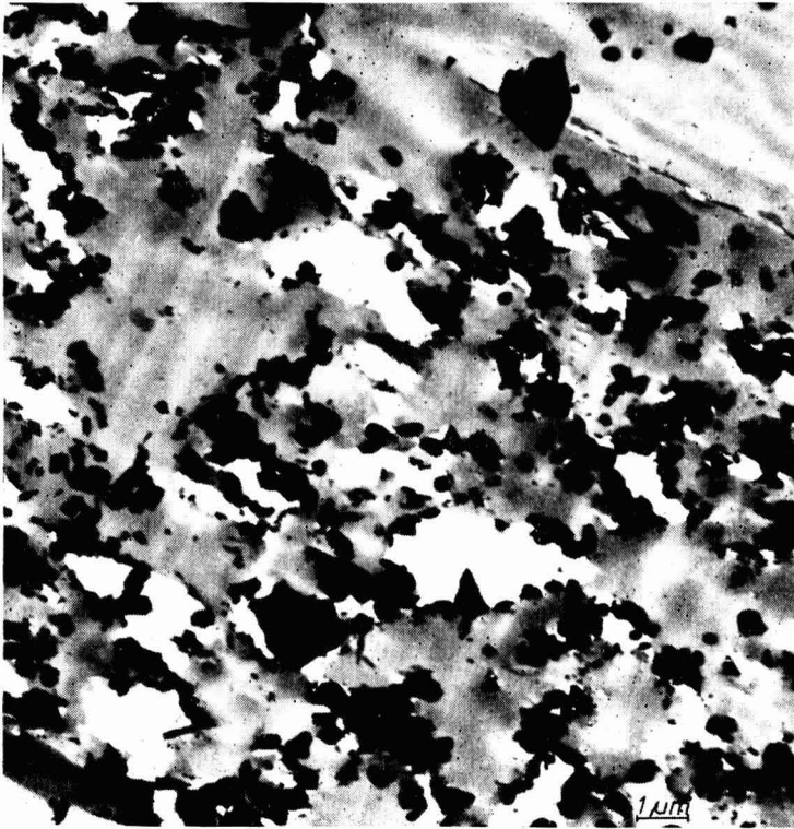
Fig. 17. Cross-section ( \times 9,000 ) of an epoxy resin/red lead film ( \lambda_p = 0.3 )
