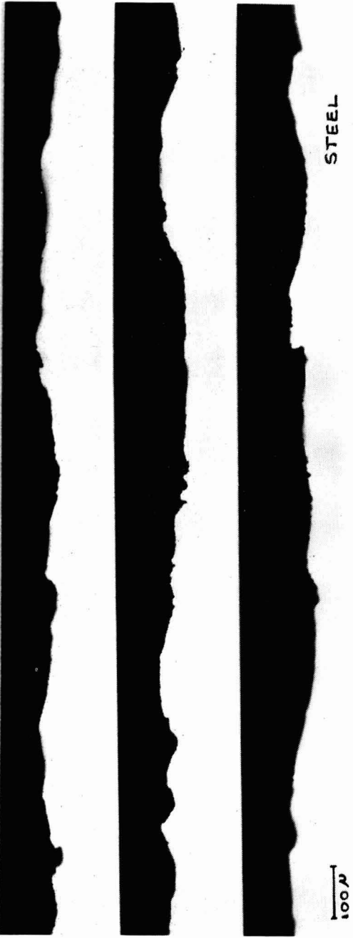
Fig. 9a. Photomicrograph of profile of steel plate shot blasted with 25 mesh steel shot to Swedish Standard Sa3
