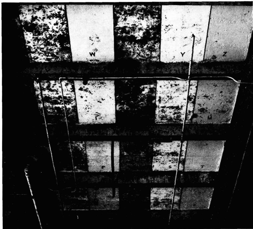
Fig. 1. Test area on ceiling over bottle washing machine in brewery, 11 months after painting with formulations detailed in Table 1
