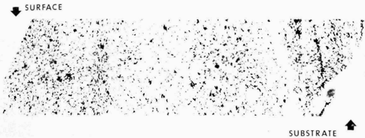
Fig. 5. Montage of electron micrographs of \text{TiO}_2 pigmented acrylic powder coating
