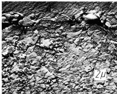
Fig. 7. Electron micrograph of the interfacial region after the top layer of a modified alkyd paint (A) has penetrated into cavities in the nitro-cellulose (N) undercoat
