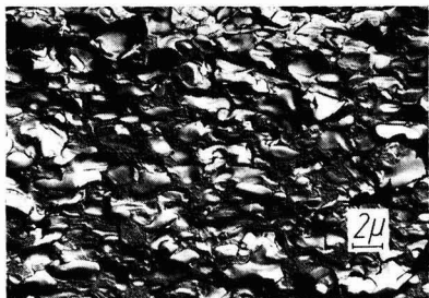
Fig. 5. Electron micrograph of a film made from a solution of forty per cent non-solvent in the solvent blend
