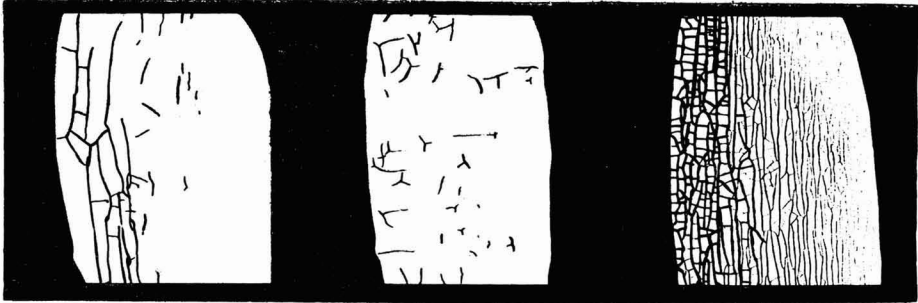
Fig. 9. From left to right: Type A, Type E and Type J fractures, based on reference standards produced by Verfinstituut TNO, Holland
