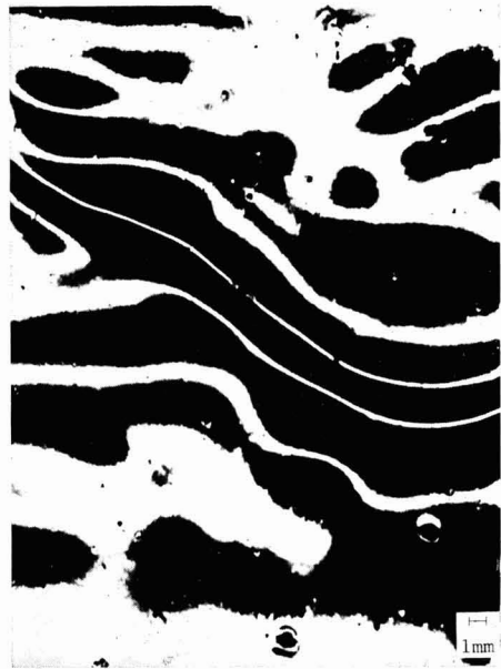
Fig. 14. Schlieren images of sagging paint film. (a) Knife edge schlieren stop aligned parallel to sag front so as to just cut off deflected light. (b) Slit schlieren stop aligned parallel to sag front so that light deflected in up and downward directions is cut off
